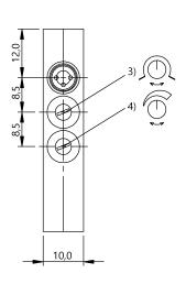
1) Output function, 2) Optical axis, 3) Light-on/dark-on, 4) Sensitivity
